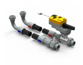
The flexible hoses package for RDHX Pro connects the cooling device to facility water system. The high quality EPDM hoses perform with excellent chemical stability with typical water and glycol based cooling media. The steel reinforcement provides extended pressure capability with rated nominal pressure 5 bar and minimum burst pressure 20 bar, while the external layer protects the hoses from mechanical stress and damages.
