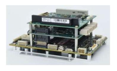
Diamond s EMM-8EL-XT PCIe/104 module offers 4 or 8 RS-232/422/485 serial ports with or without optoisolation.
