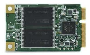
The SATA DOM module plugs onto a SATA connector and is fixed in place with a screw for shock and vibration resistance.
