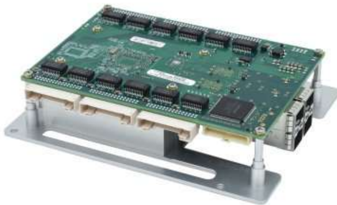
EPS-24G4X Ethernet switch with conduction cooling used in SabreNet-24000
