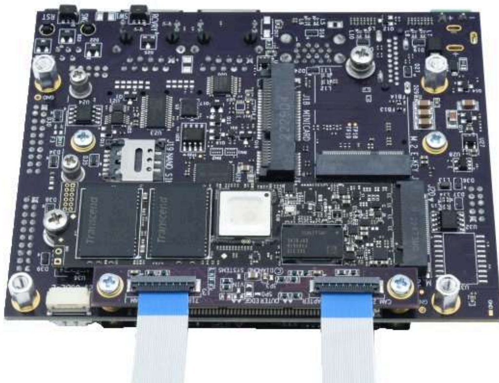
Bottom side with dual 4-lane CSI adapter board installed
