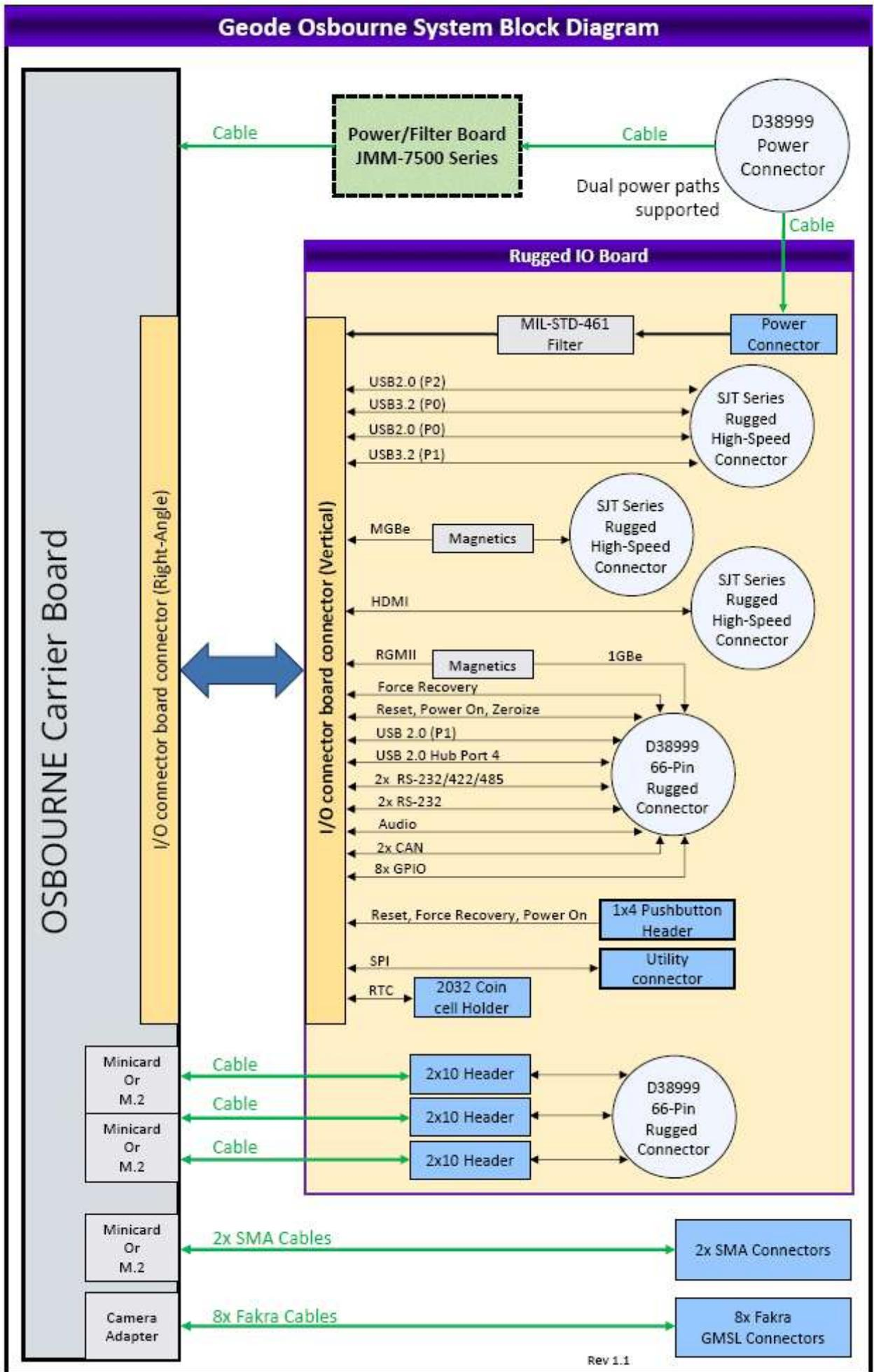
The Osbourne carrier board includes 2 minicard sockets and an M.2 E-Key socket for installing I/O and connectivity expansion modules. The Panel I/O board provides 3 connectors to bring out the I/O from installed expansion modules without requiring enclosure redesign. It has capacity for up to 60 I/O signals. Two SMA connectors are also provided on the front face of the enclosure for installed communications modules.
