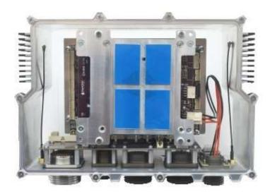
The entire system is housed in a rugged 3-part enclosure that eliminates all T joints and includes seals at all joints to ensure IP67 compliance.
