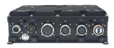
SabreCom-4 is Diamond's new rugged platform for applications requiring custom I/O. Three connector positions are provided to support standard I/O options as well as customer-specific I/O. High-speed interfaces such as HDMI and USB 3.0 are supported via dedicated connectors. I/O expansion can be provided by a combination of PCIe/104 and PCIe minicard I/O modules.
