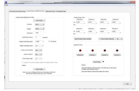
BusWorks XT software (download free from www.acromag.com) allows you to configure I/O modules offline with USB, save the file, and download settings into units later, at your convenience.
