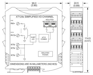
16-channel single-ended analog voltage input ◆ Modbus TCP/IP, Ethernet/IP, Profinet, or i2o communication
