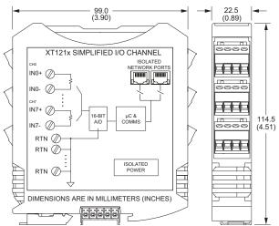
8-channel differential analog current input • Modbus TCP/IP, Ethernet/IP, Profinet, or i2o communication
