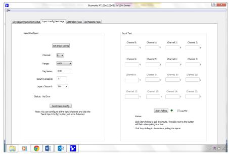
BusWorks XT software (download free from www.acromag.com) allows you to configure I/O modules offline with USB or save the configuration file and download settings into units later at your convenience.
