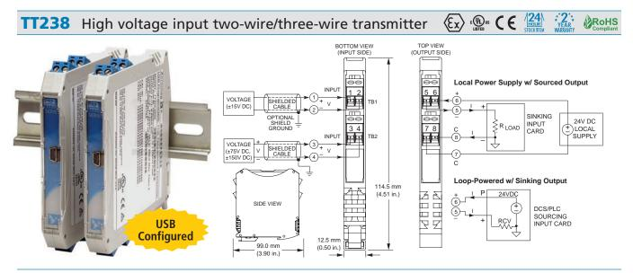
Multi-range ±15V, ±75V, or ±150V input ◆ 4-20mA output (sink/source) ◆ 12-32V DC loop/local power
