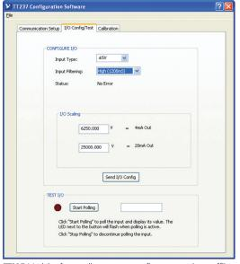
TT237 Model software allows you to configure transmitters offline. save the file, and download into units later, at your convenience.
