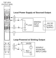
Multi-range ±1V, ±5V, or ±10V input ◆ 4-20mA output (sink/source) ◆ 12-32V DC loop/local power
