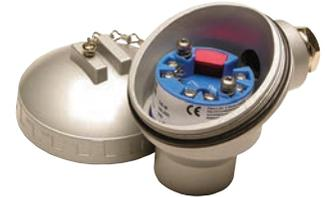
Thermocouple (8 types) or  $\pm 100\text{mV}$  input ◆ 4-20mA output ◆ 1500V isolation ◆ Loop-powered
