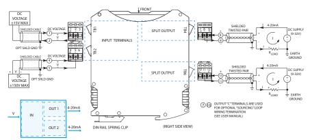
Multi-range ±15V, ±75V, or ±150V input ◆ 4-20mA outputs (sink/source) ◆ 7-32V DC loop/local power
