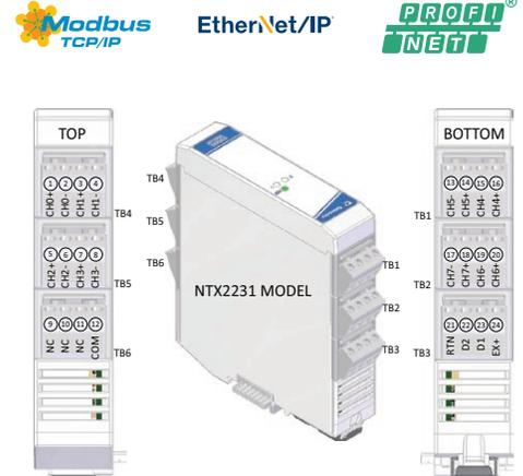
8 differential voltage inputs ♦ 2 discrete I/O ♦ Ethernet I/O plus Expansion I/O ♦ Multi-protocol support
