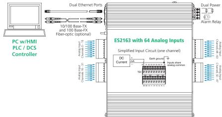
64-channel single-ended analog current input ◆ Modbus TCP/IP or UDP/IP communication
