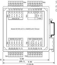
Standard model includes cage clamp terminal blocks. Optional terminals are available.
