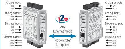
Acromag's i2o technology allows modules to talk directly to another module across any Ethernet media without a PLC, PC, or other controller in between. Input channels on one module can write to output channels on a remote module.
