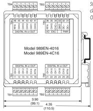
Standard model includes cage clamp terminal blocks. Optional terminals are available.
