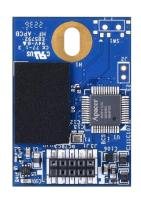
In terms of flash management, UV110-UFM2 adopts the latest page mapping file translation layer and comes with various implementations including power saving modes, wear leveling, flash block management, power failure management, S.M.A.R.T., Hyper Cache technology and SMART Read RefreshTM. With cost-effective design, better performance and increased reliability, UV110-UFM2 is well suited for embedded flash storage applications offering new and expanded functionality.
