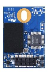
In terms of flash management, UV110-UFM1 adopts the latest page mapping file translation layer and comes with various implementations including power saving modes, wear leveling, flash block management, power failure management, S.M.A.R.T., Hyper Cache technology and Smart Read Refresh™. With cost-effective design, better performance and increased reliability, UV110-UFM1 is well suited for embedded flash storage applications offering new and expanded functionality.
