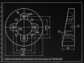
TK048.323 10° angle adapter module is made of AISI 304 quality stainless steel material and is a module that provides ergonomic use to the panels. With its high sealing feature (IP66), it can be easily used in working areas with liquid contact. The outer surface of the module is satined surface treated and sent ready for use. This product is used together with TK048.320 module.
