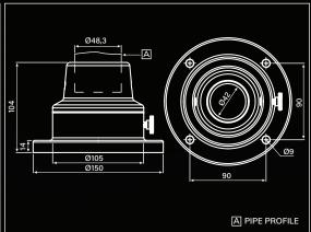
TK048.610 Top mounting module vertical outlet is a top mounting movable return module made of AISI 304 quality stainless steel material. It is fixed with four connection bolts. With its high sealing feature (IP66), it can be easily used in working areas with liquid contact. The outer surface of the module is satined surface treated and shipped ready for use. It is used with stainless steel pipe profiles with an outer diameter of 48.3 mm.
