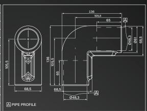
TK048.420 Corner turn module is a 90° fixed turning module made of AISI 304 quality stainless steel material. It is fixed with four connection bolts. With its high sealing feature (IP66), it can be easily used in liquid contact working areas. The outer surface of the module is satined surface treated and shipped ready for use. It is used with stainless steel pipe profiles with an outer diameter of 48.3 mm.
