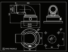
TK048.600 Top Mounted Module Corner Outlet is a top mounting movable turning module made of AISI 304 quality stainless steel material. It is fixed with four connection bolts. With its high sealing feature (IP66), it can be easily used in liquid contact working areas. The outer surface of the module is satined surface treated and shipped ready for use. It is used with stainless steel pipe profiles with an outer diameter of 48.3 mm.
