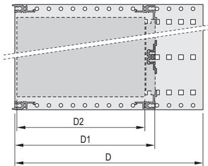
D=overall depth, D1=insertion depth,
