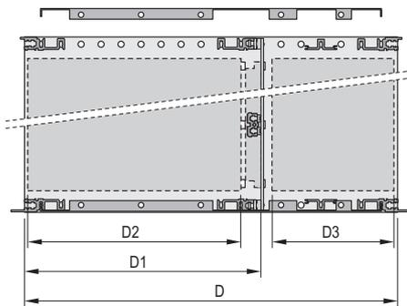
D = overall depth, D1 = insertion depth,
