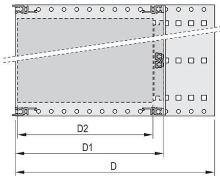
D = overall depth, D1 = insertion depth,
