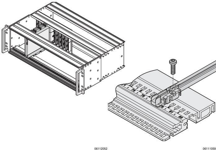
Guide rails form the interface between the subrack mechanics and the assemblies (boards, plug-in units, frame type plug-in units, drive unit modules, ...).
