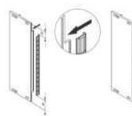
EMC gasket stainless steel, for U-shaped front panel
