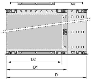
D = overall depth, D1 = insertion depth,
