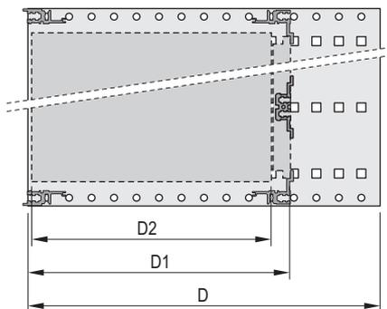
D = overall depth, D1 = insertion depth,
