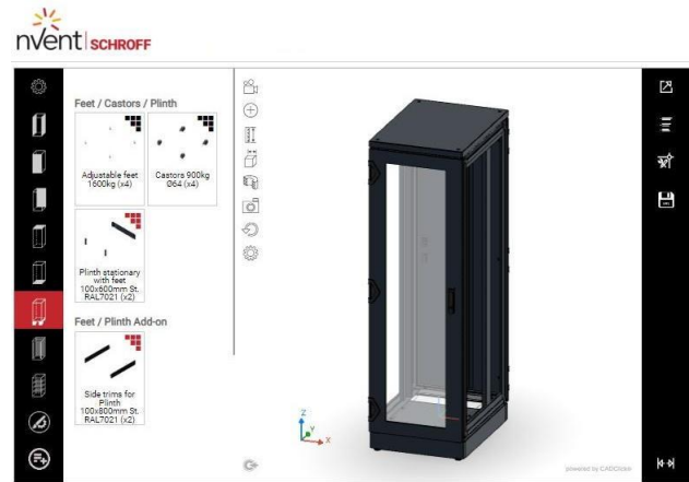
2. Select the external cladding parts like: Doors, side panel, top cover, base plate and plinth
