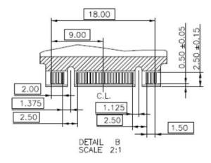
Note: the top side thickness is without the heat spreader. Heat spreader adds approximately 0.4mm to the thickness.
