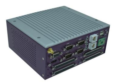
The MIDI-Aries series is based on our rugged, I/O-rich **Aries SBC**. This board features the Intel "Bay Trail" E3845 CPU with an extensive set of PC I/O such as dual gigabit Ethernet, 4 multiprotocol RS-232/422/485 serial ports, and 2 USB 2.0 ports. The PC/104-Plus and PCIe MiniCard sockets enable easy I/O expansion with hundreds of I/O modules. Expansion is made easier with the prefab connector cutouts hidden behind a removable panel along the lower front edge.
