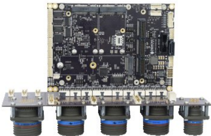
Internal view showing JASPER COM Express carrier with expansion sockets direct-connected
