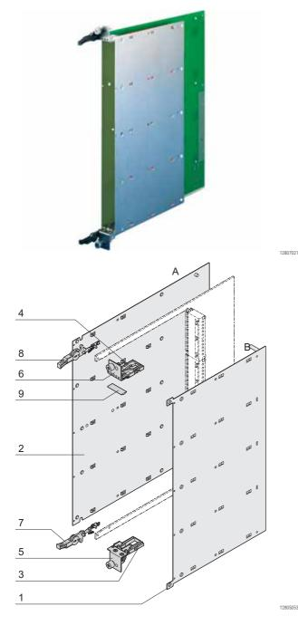
• Mechanics for cutaway carrier board (carrier **without** struts, guide rails, ESD clips, for individual placement)
