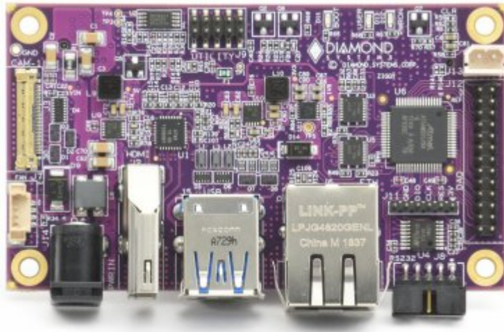
Ziggy Carrier for Jetson TX2/TX2i (2.0x3.4" / 50x87mm) Top View
