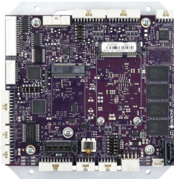
Saturn rugged SBC with E3940 CPU and data acquisition
