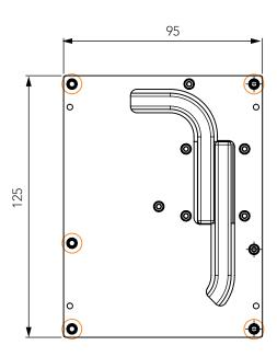
M2.5 x 11 mm threaded standoff for threaded version or ø2.7 x 11 mm non-threaded standoff for borehole version
