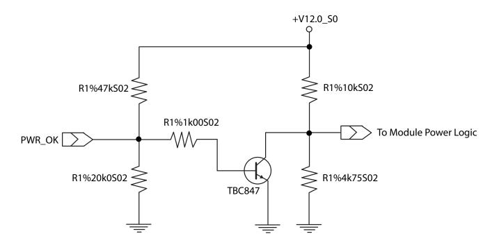
The voltage divider ensures that the input complies with 3.3V CMOS characteristic and also makes it possible to use the module on carrier board designs that do not drive the PWR\_OK signal. Although the PWR\_OK input is not mandatory for the onboard power-up sequencing, it is strongly recommended that the carrier board hardware drives the signal low until it is safe to let the module boot-up.
