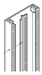
• Required for fitting of cable retention rails or slide rails on stationary 19" lab rack
