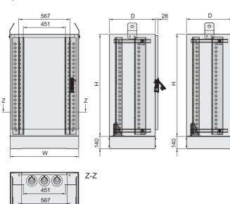
Dual access Height of door opening = H - 270 mm; width of door opening = W - 100 mm
