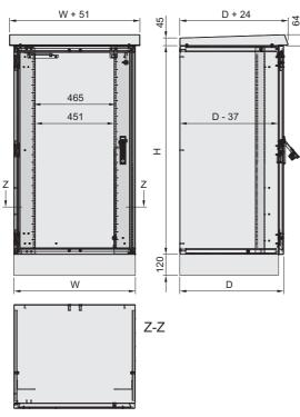
Drawing shows version with plinth Door opening height = H - 75 mm; door opening width = W - 75 mm
