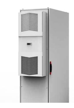
Slim Fit air conditioners are specially designed and developed to meet the requirements of industrial customers. Slim Fit air conditioners are easy to specify and ready to use. Available with a cooling capacity range from 300W to 4000W. All units are tested for IP54 for an operating temperature range 10°C to 55°C.
