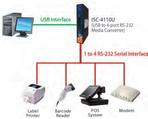
Connections of USB to Serial Media Converter
