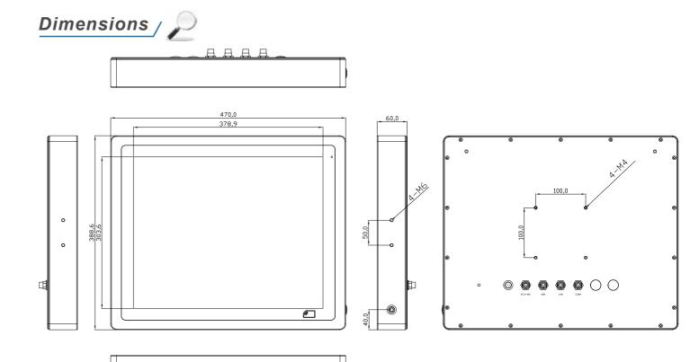
Mechanical 304 Stainless steel chassis(default), 316 Stainless steel Construction chassis(optional) VESA mount 100 x 100, Yoke mount for optional Mounting IP Rating Total IP66/IP69K 470 x 388.6 x 60 mm Dimensions
