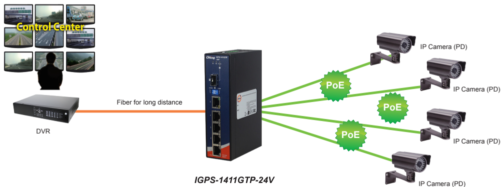
Connections of Ethernet devices
