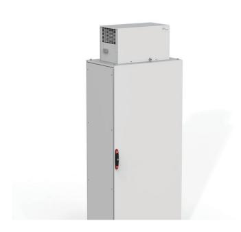
This roof cooling unit, CUH, with a IP 54 protection degree, provides cooling, either to one enclosure or to a complete assembly, depending on the cooling requirements and desired energy consumption level. It is placed on top of the enclosure and is perfect when there is not enough space on the door or side panels.
