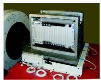
Shock and vibration resistant in all three axial directions
