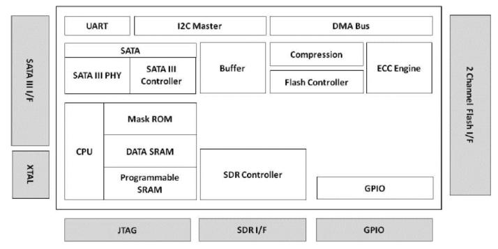
Figure 1: APRO SLC Industrial Rugged Metal 2.5" SATA III SSD PHANES-K Series block diagram
