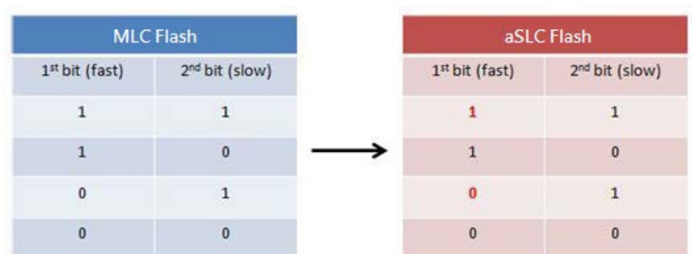
Figure 2: The concept of APRO aSLC Mini SATA III Module (mSATA) PHANES-HR Series
