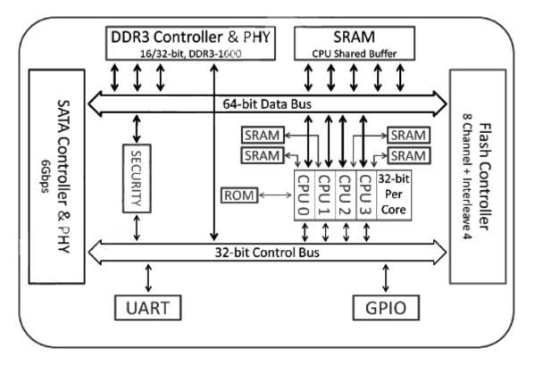
Figure 1: APRO MLC Rugged Metal 2.5" SATA III SSD PHANES-HR Series block diagram
