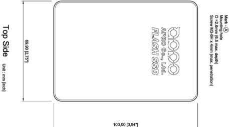
Figure 3: APRO MLC Rugged Metal 2.5" SATA III SSD PHANES-HR Series Dimension
