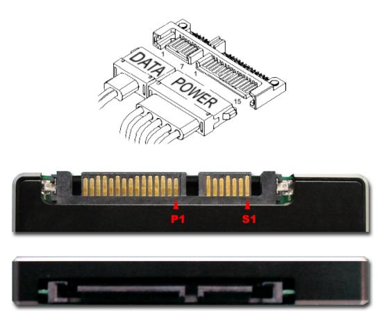
Figure 4: The connectors of APRO MLC Rugged Metal 2.5" SATA III SSD PHANES-HR Series
