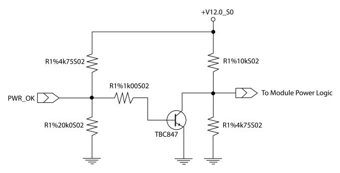
The voltage divider ensures that the input complies with 3.3V CMOS characteristic and also allows for carrier board designs that are not driving PWR\_OK. Although the PWR\_OK input is not mandatory for the onboard power-up sequencing, it is strongly recommended that the carrier board hardware drives the signal low until it is safe to let the module boot-up.
