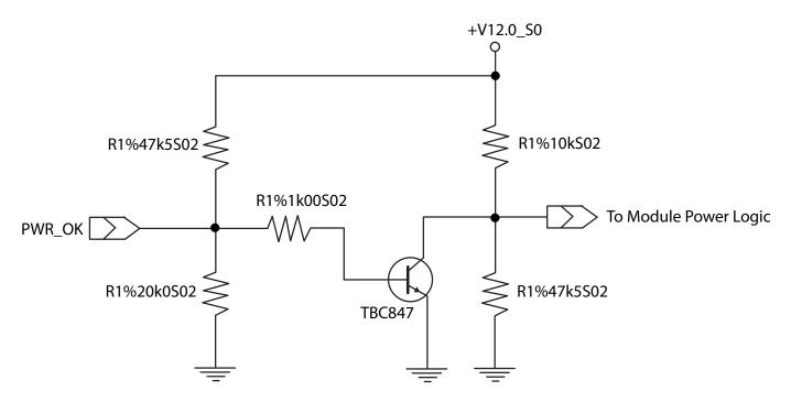
The voltage divider ensures the input complies with 3.3 V CMOS characteristic. It also makes it possible to use the module on carrier board designs that do not use the PWR\_OK signal. Although the PWR\_OK input is not mandatory for the onboard power-up sequencing, it is strongly recommended that the carrier board hardware drives the signal low until it is safe to let the module boot-up.
