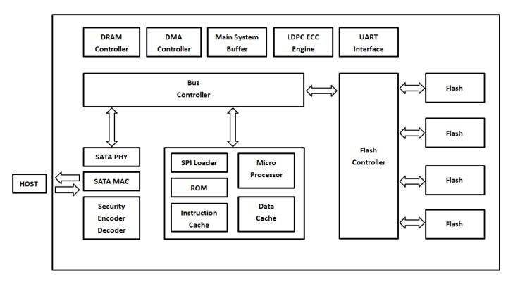
Figure 1: APRO Rugged Metal 2.5" SATA III SSD (3D-NAND Flash) MUSE-ET Series block diagram
