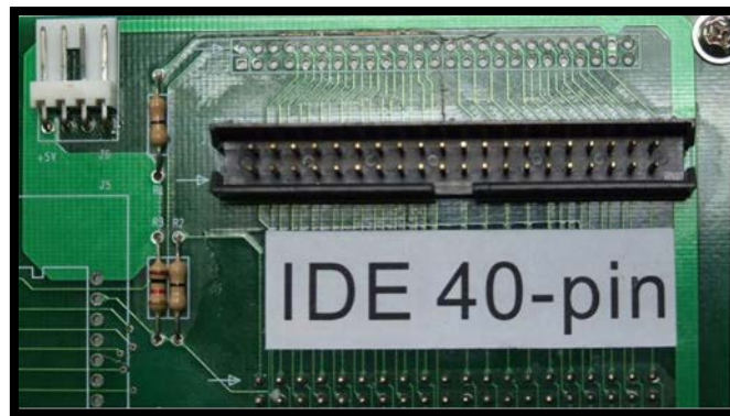
Figure 17: Intact IDE male pins on Motherboard
