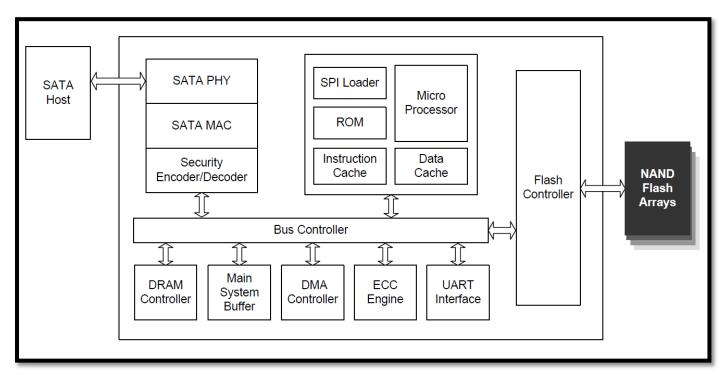
Figure 1: APRO SLC Industrial 2.5" Rugged Metal SATA III SSD HERCULES-TT Series block diagram
