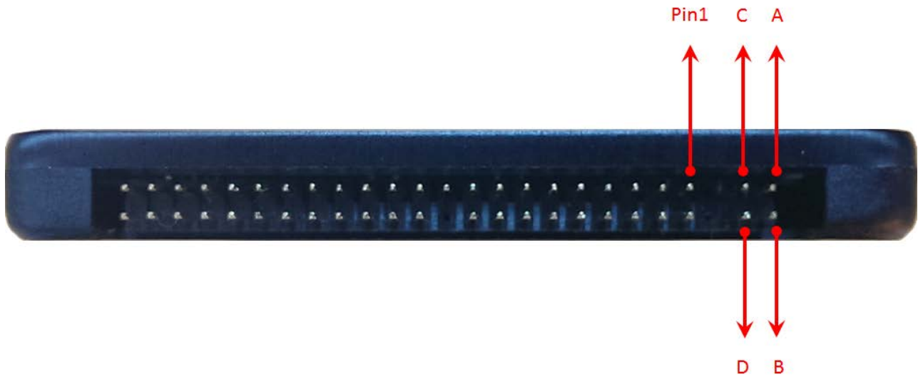
Figure 3 : The connectors of 2.5" PATA MLC SSD
