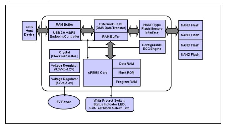
Figure 1: APRO MLC Semi-Metal USB Flash Disk Gen-5/5L HERCULES-PD Series block diagram
