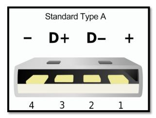
Figure 3: USB Type A Connector
