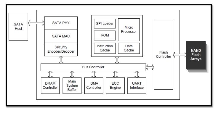
Figure 1: APRO SLC Industrial 2.5" Rugged Metal SATA III SSD BON-III series block diagram
