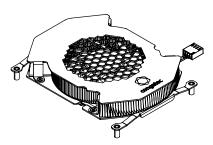
M2.5 x 10 mm threaded standoff for threaded version or ø2.7 x 10 mm non-threaded standoff for borehole version
