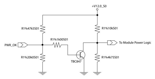
The voltage divider ensures the input complies with 3.3 V CMOS characteristic. It also makes it possible to use the module on carrier board designs that do not use the PWR\_OK signal. Although the PWR\_OK input is not mandatory for the onboard power-up sequencing, it is strongly recommended that the carrier board hardware drives the signal low until it is safe to let the module boot-up.
